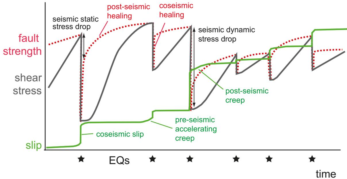
**Fig. 2.** The fault strength and shear stress on a fault patch evolve with time during the seismic cycle. Fault failure is the result of the complex feedback between the loading stress and the evolution of the fault strength with time. Pre-seismic accelerating creep might occur for some earthquakes. Post-seismic creep might be as large as coseismic slip in some fault patches. This framework renders a physically-based earthquake forecasting model an extremely challenging task.
