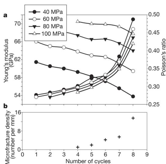
**Figure 2** | Variation of measured elastic properties with increasing microfracture damage in Westerly granite. **a**, Change in Young's modulus (increasing curves) and Poisson's ratio (decreasing curves) with increasing damage. Data are shown for stresses of 40, 60, 80 and 100 MPa. Cycle 1 was taken to a maximum stress of 80 MPa and the stress was increased by  $\sim 12$  MPa on each subsequent cycle. **b**, Increase in microfracture density with increasing damage.
